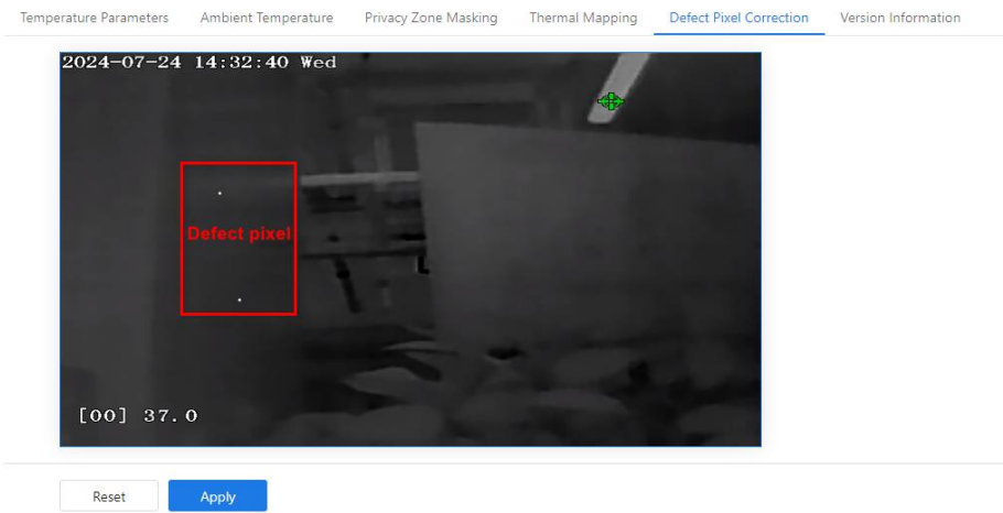
Figure 5-6 Defect pixel correction
