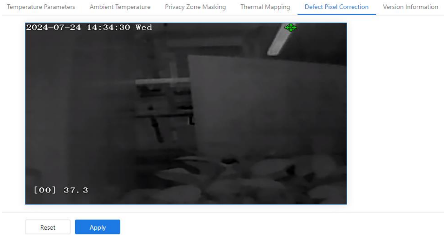
Figure 5-7 Recover Defect Pixel
