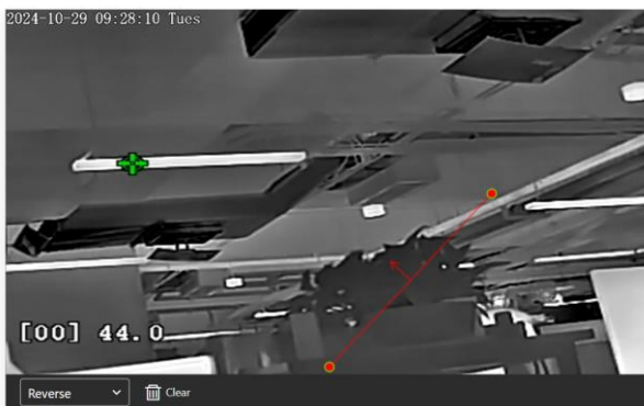
Figure 5-5 Set Single Line Crossing Line
