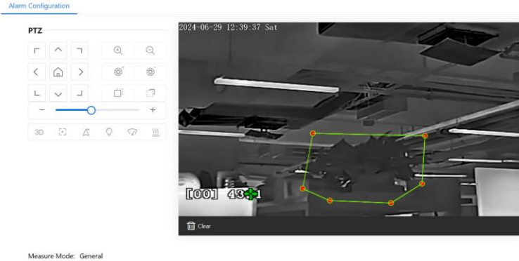
Figure 4-8 Temperature Area Setting Interface
