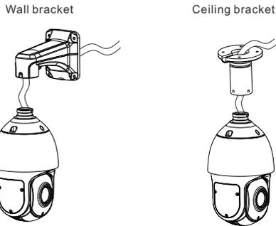
Step 3 Attach the high speed dome to the bracket, the tighten the three screws, as shown in figure 3-3.
