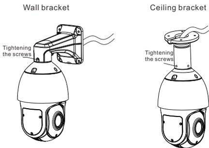
Step 4 Mount the high speed dome to the wall or ceiling and tighten the four expansion bolts on the bracket completely.
